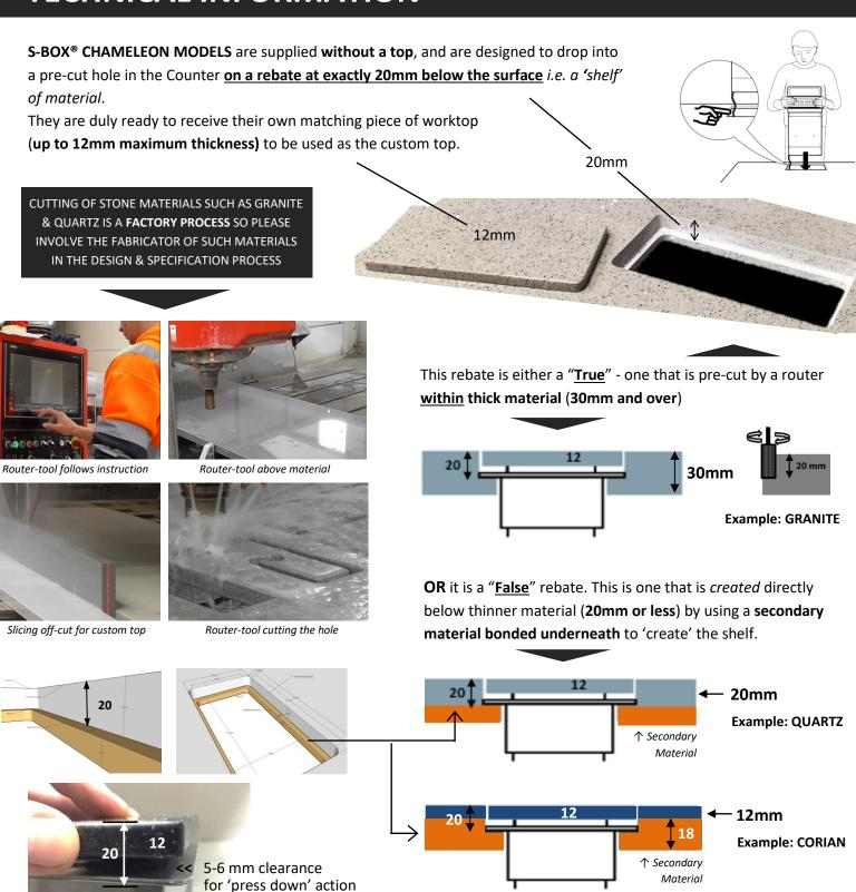
FULL INSTRUCTIONS, DATA SHEETS, CAD FILES AND CUTTING DIMENSIONS FOR ALL INSTALLATIONS ARE LOCATED AT: https://www.the-sbox.com/tech-data/
