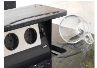
NEC 2.2 litre (½ Gallon) Saline Liquid Spill Test 406.5 (E)
