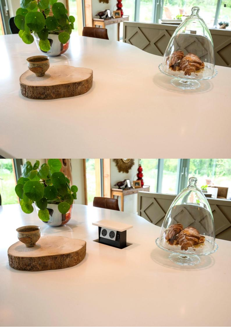
S-BOX™ CHAMELEON MODELS are supplied with a special 'any-radius' black collar. This is pre-set and fixed for installation of the unit <u>at -20mm below the surface on a rebate shelf</u> — one that is pre-cut within (or 'created' below) the counter material. The unit is therefore ready to receive a piece of worktop material <u>up to 12mm thick maximum</u> — to be used as the unit's top.
