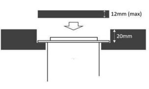
S-Box® Chameleon uses a 12mm (max) piece of your work-top material to create a blended and camouflaged installation.
